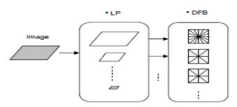
The structural design of contourlet via laplacian pyramid and directional filter is as follow:
