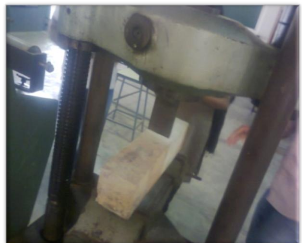
Figure 4: Typical Flexure Failure pattern of concrete Cubes
