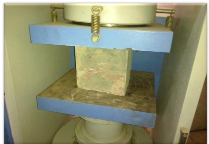
Figure 2: Typical compressive failure pattern of concrete Cubes
