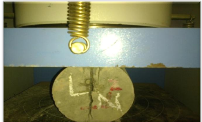
Figure 3: Typical Tensile Failure pattern of concrete Cubes
