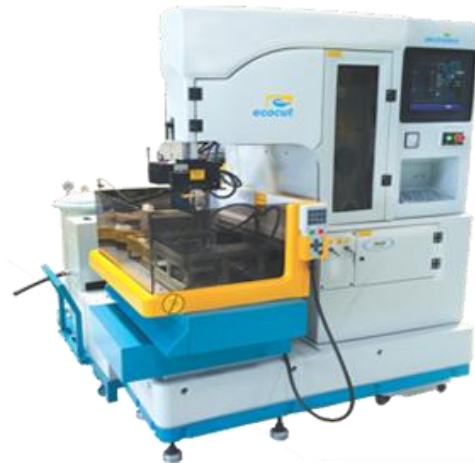
Fig 1. Schematic representation of WEDM [1] and M/c tool used
